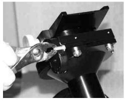
7) Add plastic washer (B) and threaded spacer (C) onto protruding set screw. Tighten with pliers.
