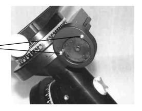
9) Put two allen head mounting screws (E) into the servo motor, slide into the gear cover, and rotate until you feel the screws drop into the threaded holes. Tighten.
