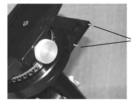
5)Thread set screws (A) into motor mount holes until they protrude out 3/8".
